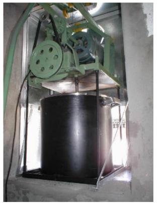
Fig. 3. Cooking pot inside its cage with mixer put on the cooking place (without insulating panels)
