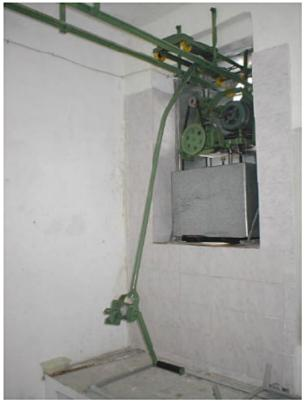
Fig. 4. Cooking pot in cooking position (with insulating panels) and elevating system
