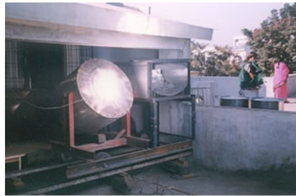
Photo shows the storage cooker and the direct cooker on rails.
